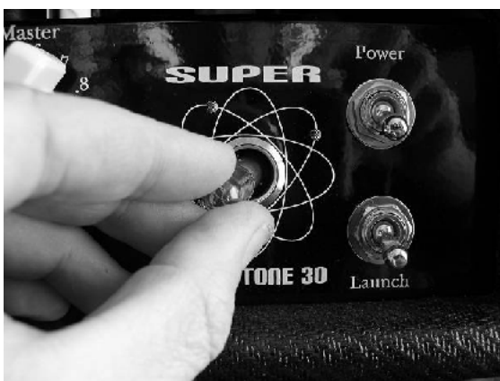
5 Align bayonets, push in, turn right to lock.
