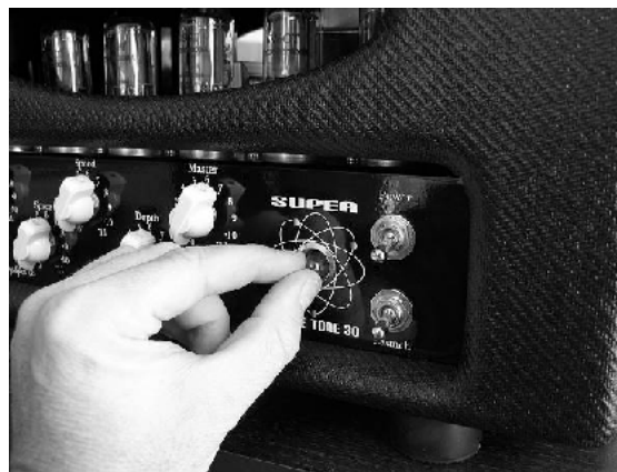
2 Push bulb in, rotate left to release bayonets.
