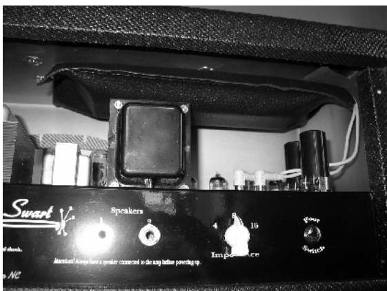
3 See Reverb Tank at top right within pouch
