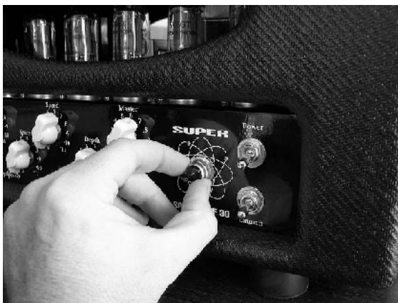
1 Turn the knurled base counter clockwise to remove.
