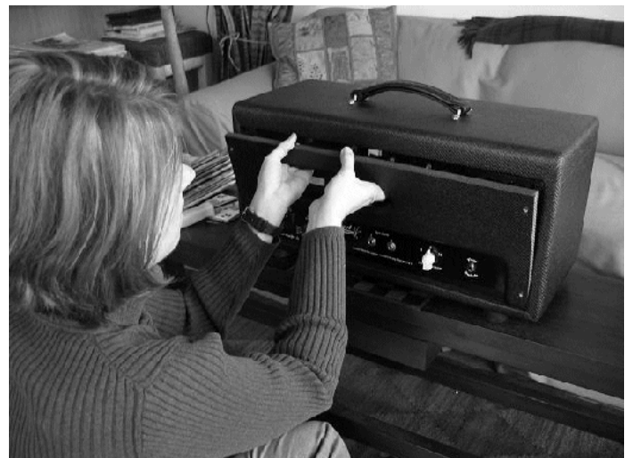
Step 3: Tell poor sap to make sure to grasp the panel as above, carefully pulling out from top first.
