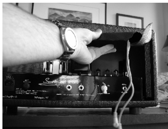
6 Carefully swivel tank and pouch out, maneuvering over the Output transformer
