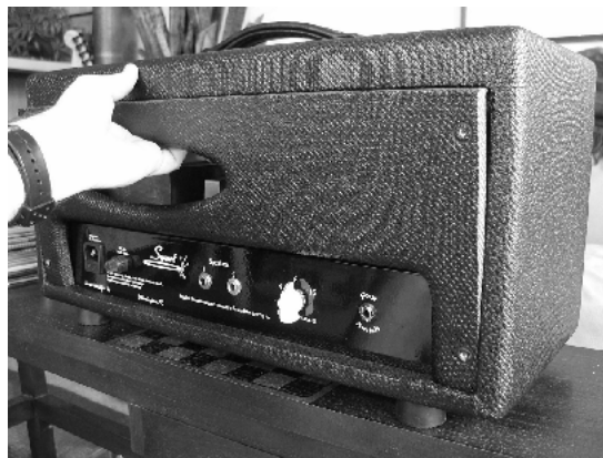
2 Remove panel as seen above, pulling out top first.
