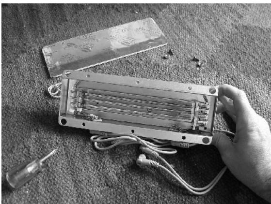
11 See exposed tank springs along with wiring to jacks
