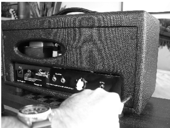
1 Unplug IEC and remove the 4 Phillips Head Screws
