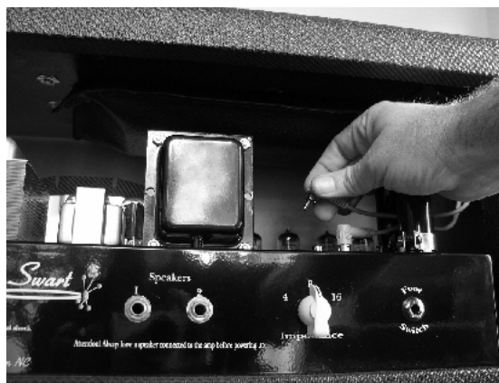
4 Remove Tank leads from chassis RCA's (output/input)
